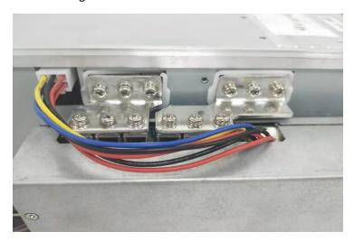
Please insert the 6-pin plug into the matching socket.
