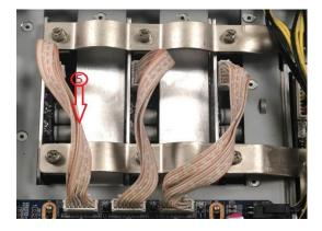
(3) Fan connection. Connecting with fan cable(by 4PIN connector).
