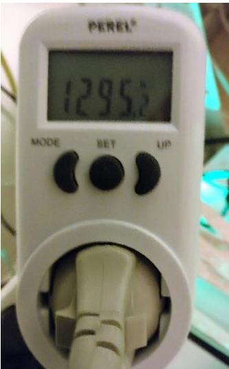
Figure 40 Power consumption measurement, when the voltage offset value is +1.
