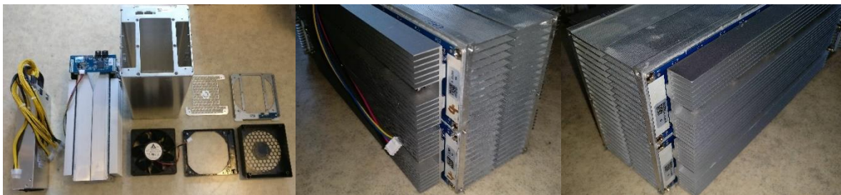
Figure 9 AvalonMiner 821 disassembled, picture set 1.
