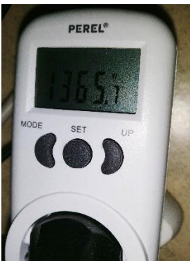
Figure 59 Power consumption measurement, when the voltage offset value is -1.
