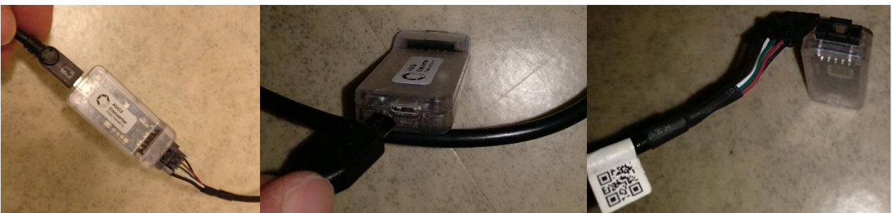
Figure 37 Connecting cables to the AUC3 Converter.
