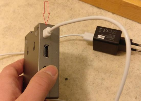
Figure 35 Connecting 5 VDC power to the controller unit.
