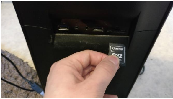
Figure 29 Integrated SD card reader in my PC case front panel.
