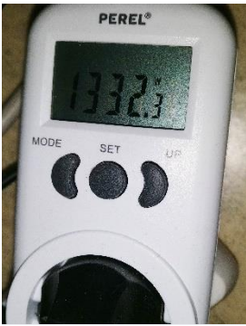
Figure 58 Power consumption measurement, when the voltage offset value is -2.
