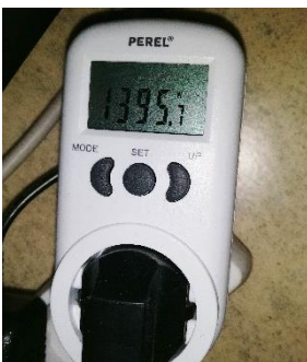
Figure 61 Power consumption measurement, when the voltage offset value is +1.
