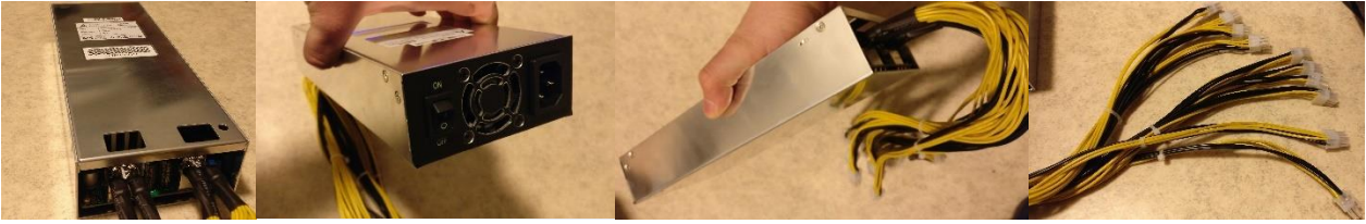
Figure 15 Sorcerer Power Supply Unit.
