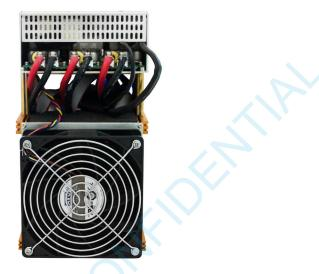
Connect the miner and the router by the Ethernet cable, then the miner can start to run after power on the miner.
