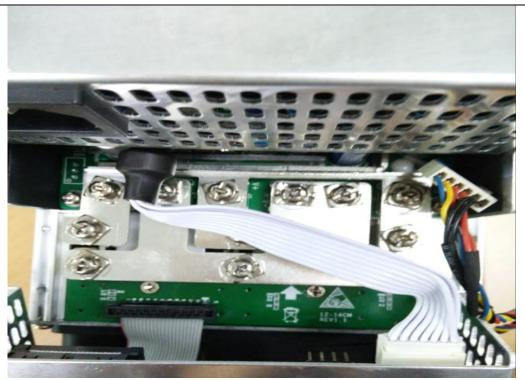
3) Unplug the power control cable and the adapter board control cable connected to the control panel as shown:
