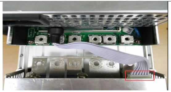
3) Unplug the power control cable on the control panel, remove the power supply, and remove the power supply:
