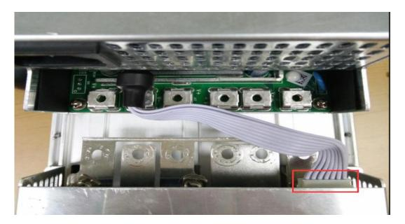
2) Then connect the 6 positive and negative terminals on the power supply to the copper row one by one, and then install 6 screws in turn. The screws should be tightened and the gasket should be aligned parallel to the edge of the copper bar to avoid short circuit burning the power supply or the power board, as shown below:
