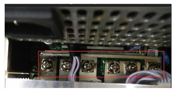
3) Finally, tighten the screws of the four fixed power supplies on the chassis, and the power supply is installed, as shown below:
