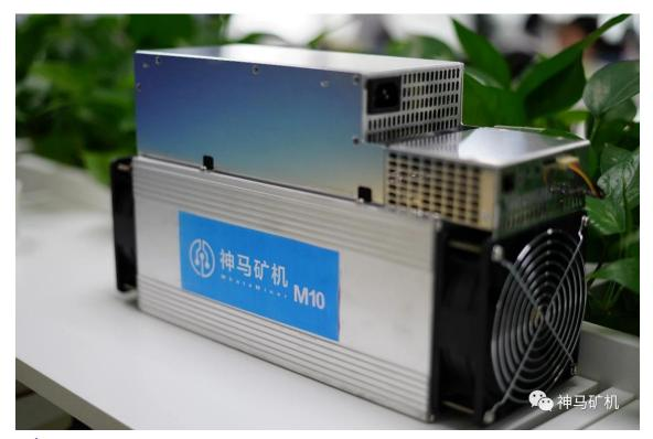
Whats Miner M10 Bitcion Mining Magic Product ParameterIntroduction as below: HashRate: 33TH/s ±5% Chip: 315pcs 16nm ASIC Power: 2145W±10% Power Rate: 65W/T ±10% Power Supply: Whats Miner Power Supply P10 (220v,2145W ±10%) Control Panel: Own Environment Temperature: -5°C~40°C Product Size: 390mm\*130mm\*220mm
