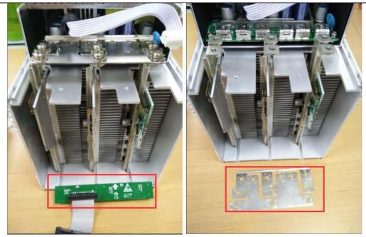
3) Extract the faulty hash board outward, as shown:
