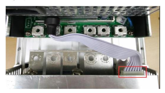
2) Then connect the 6 positive and negative terminals on the power supply to the copper row one by one, and then install 6 screws in turn. The screws should be tightened and the washers should be aligned parallel to the edge of the copper bar to avoid short circuiting the power supply or the power board, as shown below:
