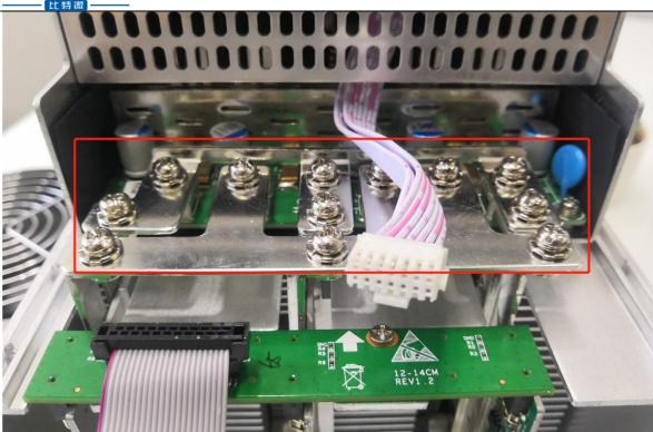
4) After the copper row is installed, the control board and the fan are installed, and the hash board is installed.
