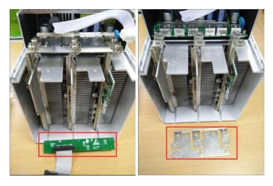
3) Extract the faulty hash board outward, as shown:
