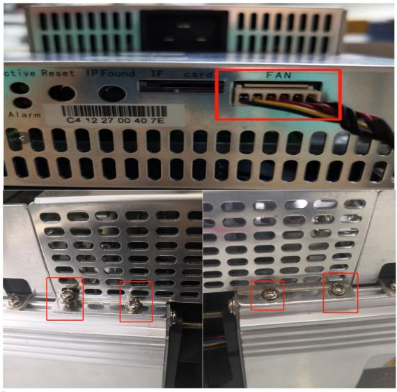
2) Unplug the power control cable and the adapter board control cable connected to the control panel as shown:
