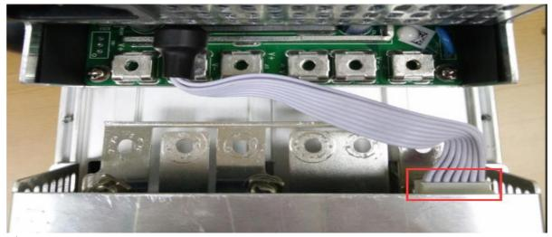
3) Unplug the power control cable on the control panel, remove the power supply, and remove the power supply:
