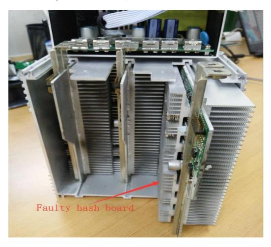
4) After taking out the hash board, record the serial number above or use WeChat "scan" to scan the power board serial number and provide it to the relevant after-sales technician, as shown:
