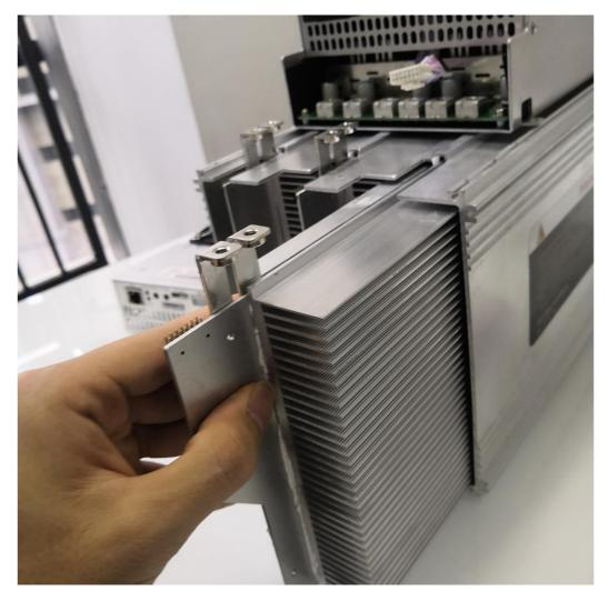
2) After installing the hash board into the chassis, first install the adapter board. The 27/29
